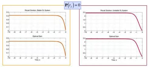
Variations in control gains are significant only in the last 10-20% of the illustrated time interval
