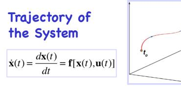
Integrate the dynamic equation to determine the trajectory from original time,  $t_{o}$ , to final time,  $t_{f}$
