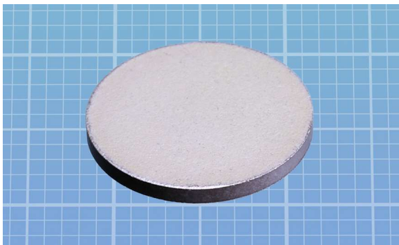
Figure 24-9 This TDK B59060A0060A010 heating element is a PTC thermistor whose resistance rises rapidly around 80 degrees Celsius. Rated for 12VDC, it is intended for automotive applications. The background grid is in millimeters.
