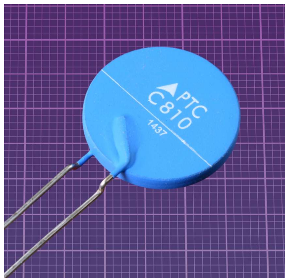
Figure 24-5 A large over-current protection PTC thermistor. The background grid is in millimeters.
