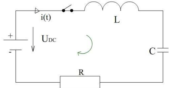
$$\left. \begin{aligned} cL \frac{d^2 u_C(t)}{dt^2} + cR \frac{du_C(t)}{dt} + u_C(t) &= U_{DC} \quad (4) \\ cL * \ddot{u}_C(t) + cR * \dot{u}_C(t) + u_C(t) &= U_{DC} \end{aligned} \right\} \text{úprava integrálu – diferenciálnych rovníc – na DR2rádu}$$
